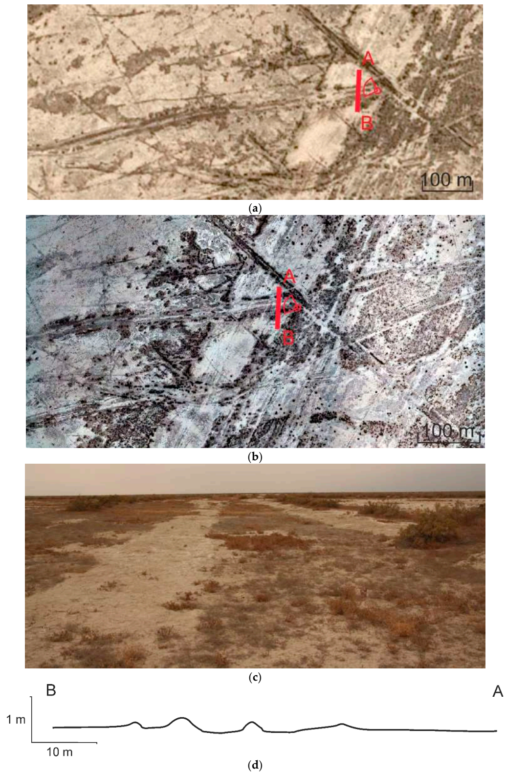
Figure 10. View of a model ice scour: (polygon 3): (a) on space imagery (WorldView-3) [42]; (b) on the ortho-photo mosaic (UAV survey); (c) ground view; (d) cross-section taken from a leveling survey. The location of the place where the ground view photo was taken is shown as a red pointer; the red line AB indicates the position of the leveling profile.
