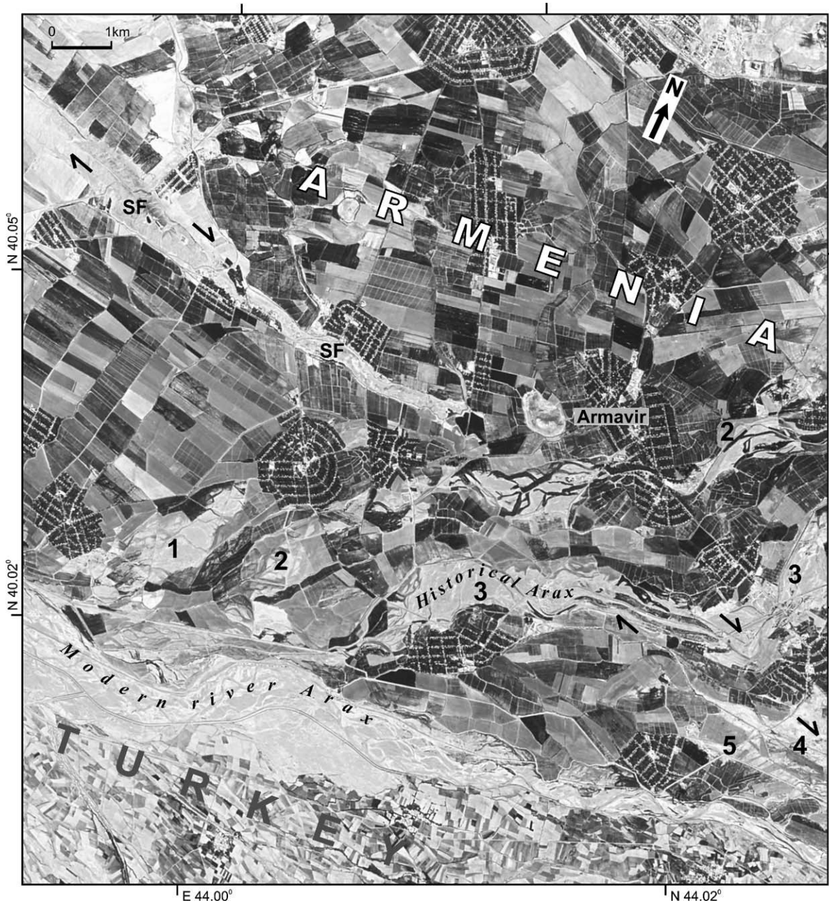
Fig. 10. CORONA satellite image of the north part of the Ararat depression (see SF in Fig. 1). There are clearly visible offsets of historical riverbeds (1, 2, 3, 4 and 5) of the Arax River, migrating southward, due to the Sardarapat fault activity (SF).
