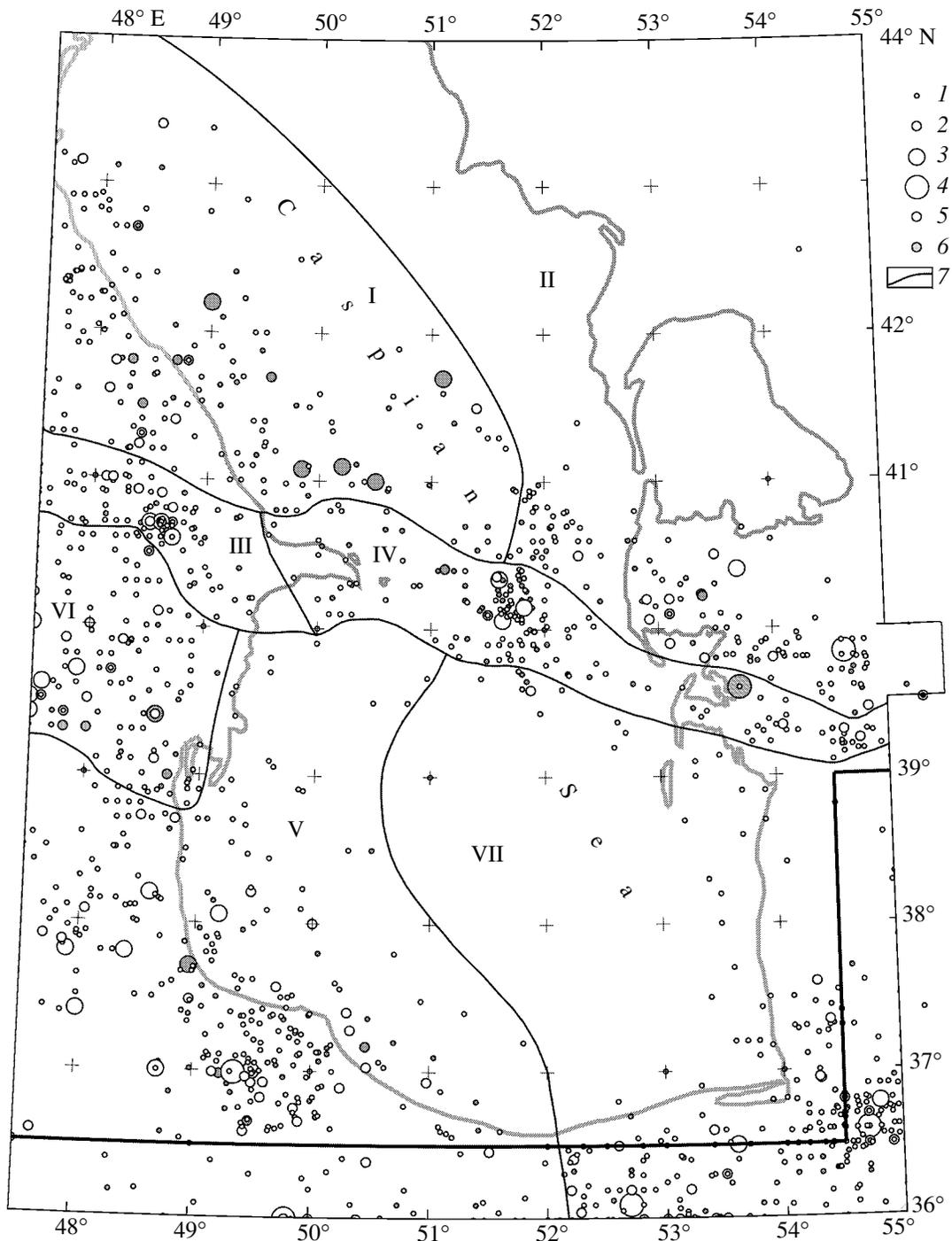
**Fig. 2.** Seismotectonic provinces I–VII and earthquake epicenters in the Caspian region: (1–4): earthquake magnitudes  $M_s$ : (1)  $<5$ ; (2) 5–5.9; (3) 6–6.9; (4)  $\geq 7$ ; (5 and 6) hypocenter depth: (5)  $\leq 33$  km; (6)  $>33$  km; (7) province boundary.
