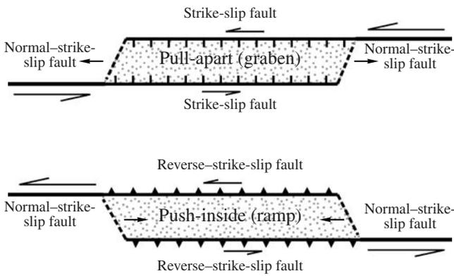
**Fig. 9.** Formation of pull-apart basins (grabens) under transtensional conditions and push-inside basins (ramps) under transpressional conditions: conceptual scheme.
