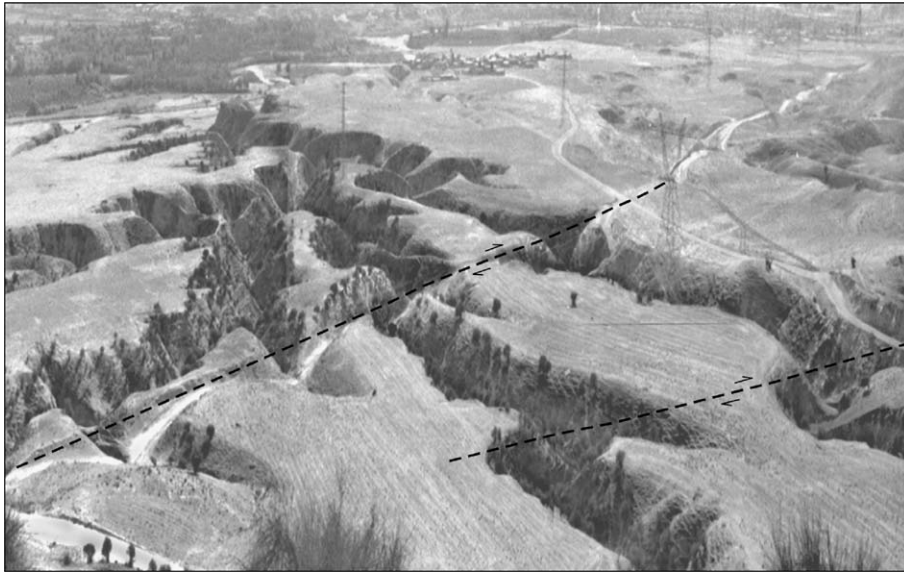
Fig. 5. Two strands of the Kazerun fault offsetting right-laterally the drainage system in the western side of the Rud-e Safid River. Photo by A.I. Kozhurin (view to the southeast).
